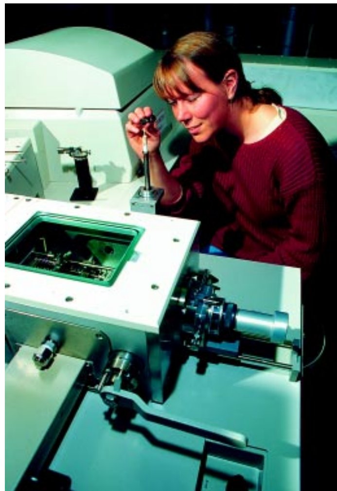
Joint Program student Elizabeth Minor repairs the sample probe on the mass spectrometer she uses to obtain molecular-level information on lipids, sugars, proteins, and other natural and synthetic substances in oceanic organic matter.
