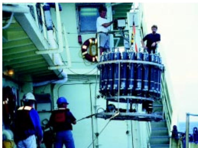
Scientists and crew swing a conductivity/temperature/depth rosette sampler into action during Oceanus Voyage 279 in summer 1996.
