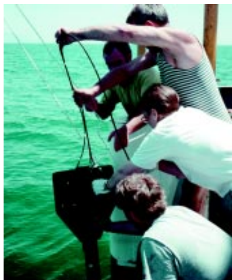
Heidi Sosik and co-workers recover a free-fall spectral radiometer used for sea-truth observations of ocean color during an expedition in the Black Sea.
